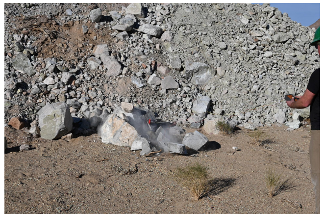
Figure 4: Post-blast results on medium boulder
