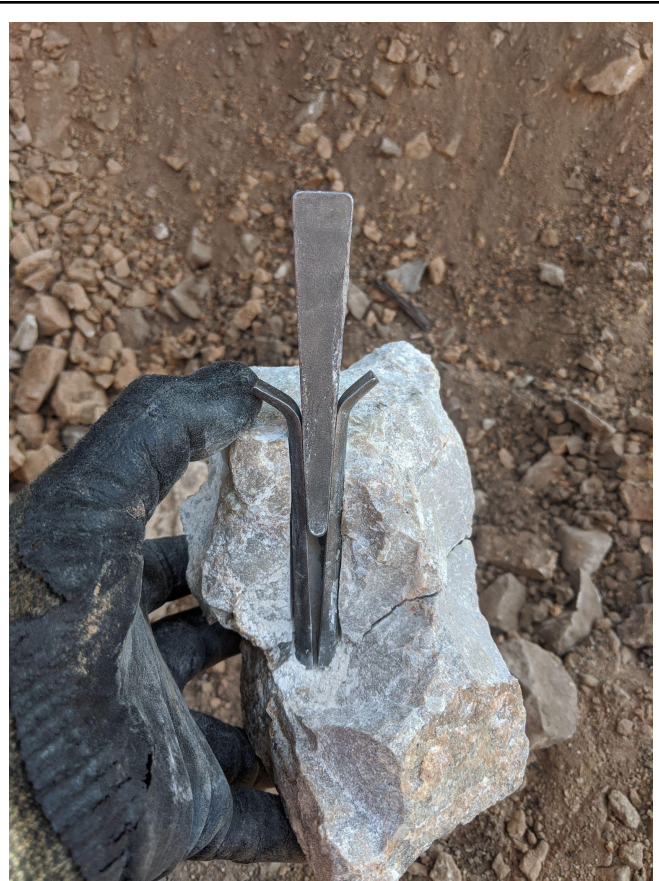
Figure 3: Cutaway view of Feather and Wedge
