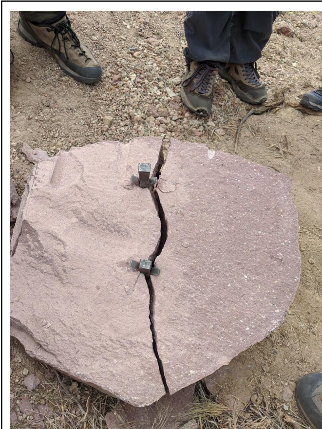
Figure 2: Feathers and Wedges in use
