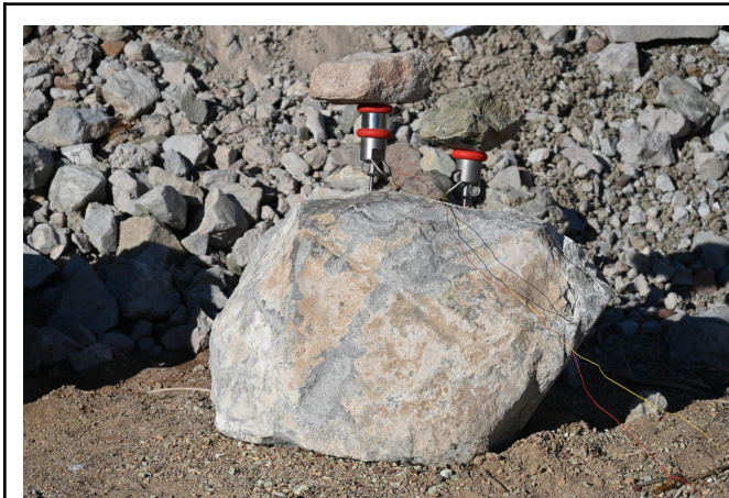
Figure 3: Two Sierra Blaster heads prepared for firing. Approximately 4 grams total explosive.
