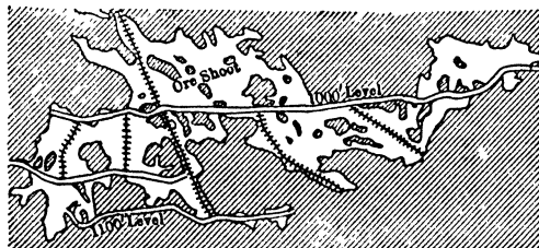
Fig 189. Part of Silver King Mine, Park City, Utah. (Aver dip, 18°; aver thickness of ore, 2.5 ft)
