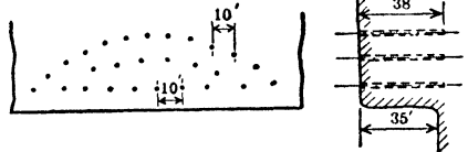
Fig 23. Arrangement of Holes for Breaking Hard Bottom
