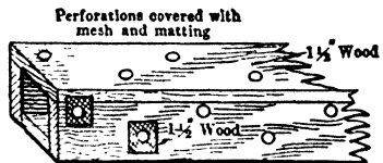
Fig 661. Drainage Launder for Sand Filling (Rand)
