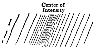
Fig 15 Sheeted Zone (Cross-sec), showing Largest Number of Cracks at Seat of Heaviest Movement
