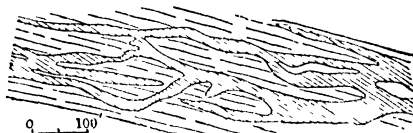
Fig 10 Irregular Replacement Orebody in Limestone (Showing Tendency toward Greatest Extent Parallel to Bedding Planes). Longit sec. After A. A. Blow
