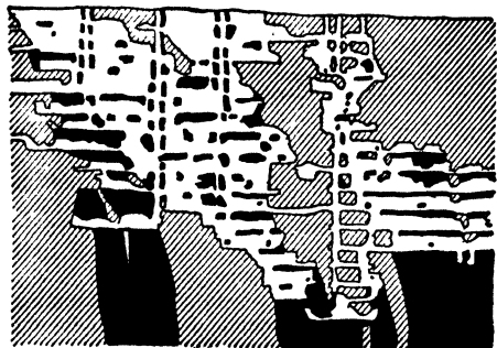
Fig 211. Underhand Stoping (Sec in plane of vein)
