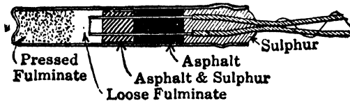
Fig 20. Electric Blasting Cap
