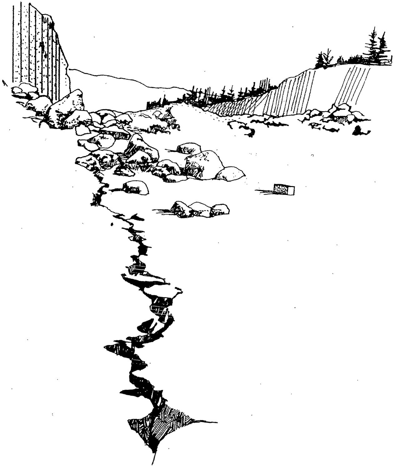
Figure 89: Crack generated by a presplit blast.
