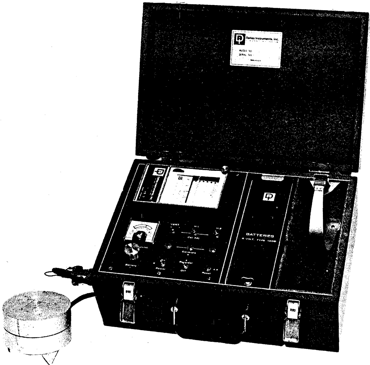
Figure 94.—Seismograph for measuring ground vibrations from blasting.
