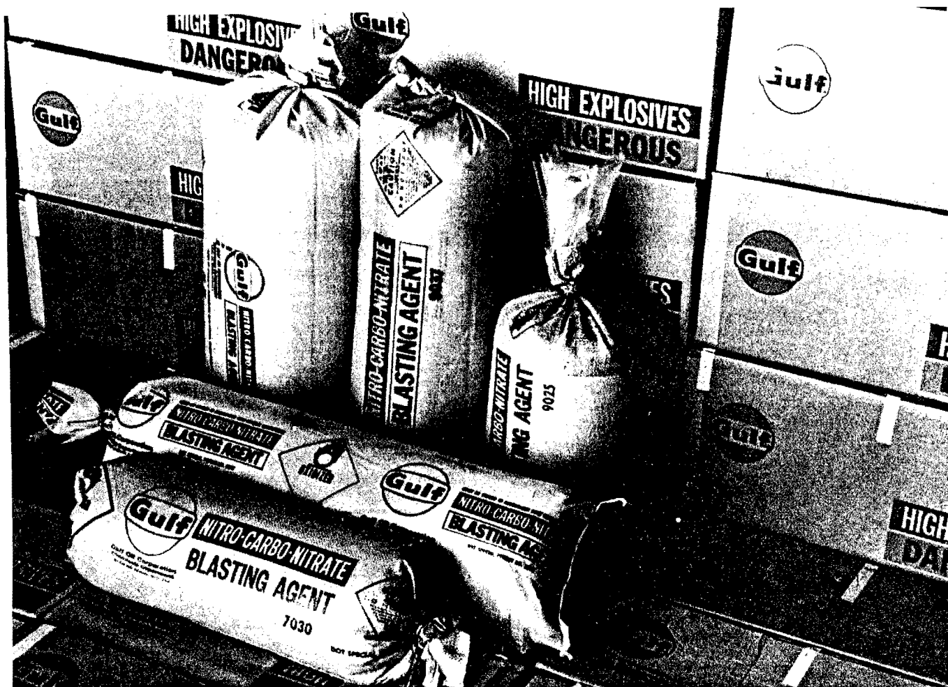
Figure 7.—Water-resistant packages of AN-FO for use in wet boreholes. (Courtesy Gulf Oil Chemicals Co.)
