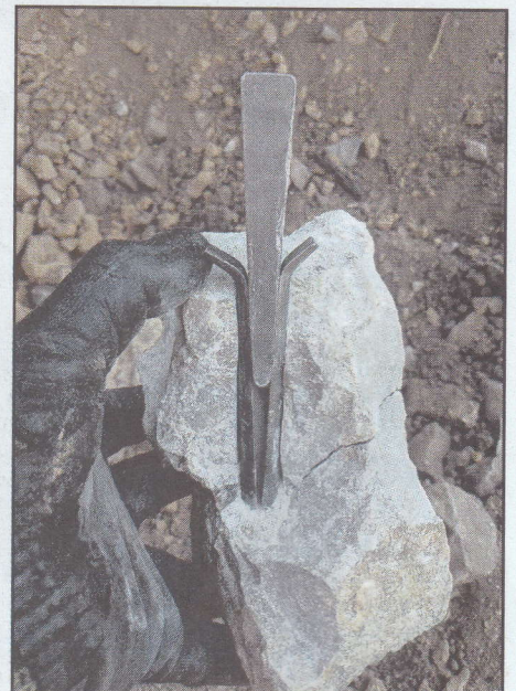
A close-up view showing how the wedge is inserted between the feathers to create a force on the rock as the wedges are hammered down. Man has been using this technique for thousands of years.
