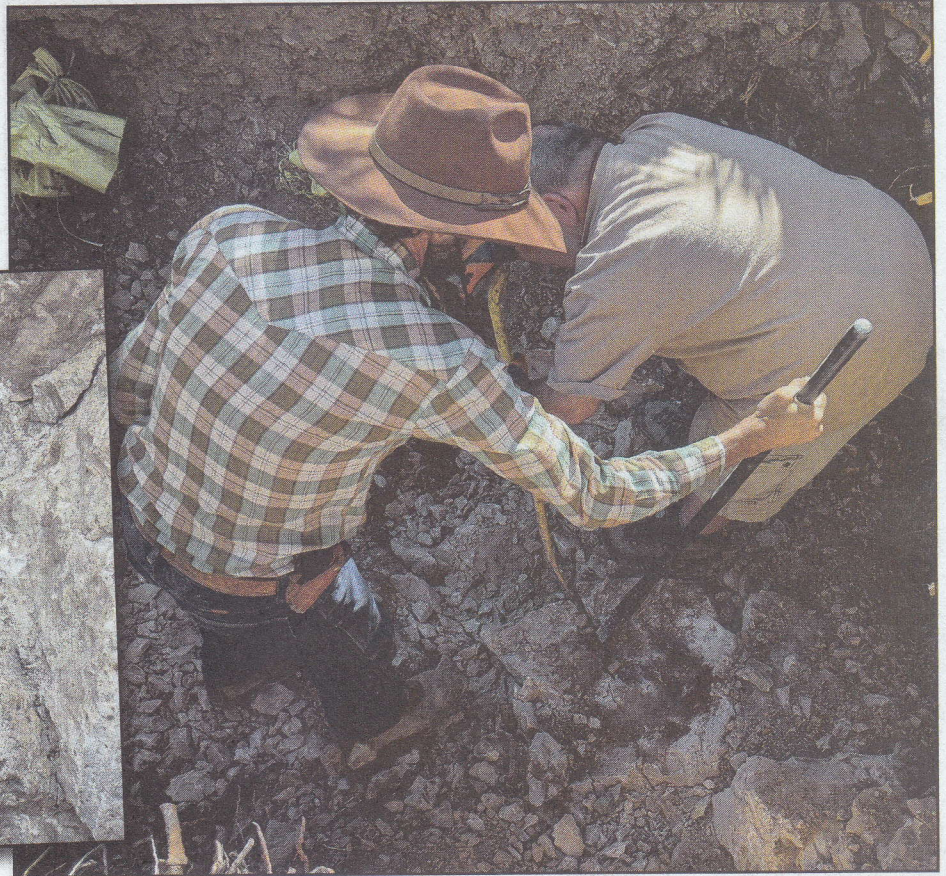
(Inset) The feather wedging process involves drilling a line of holes and then inserting a series of feather and wedge sets to create a force along the line of the holes. (Above) Keet and Tom work together to leverage the force of the pry bars to open up cracks and break the rock.
