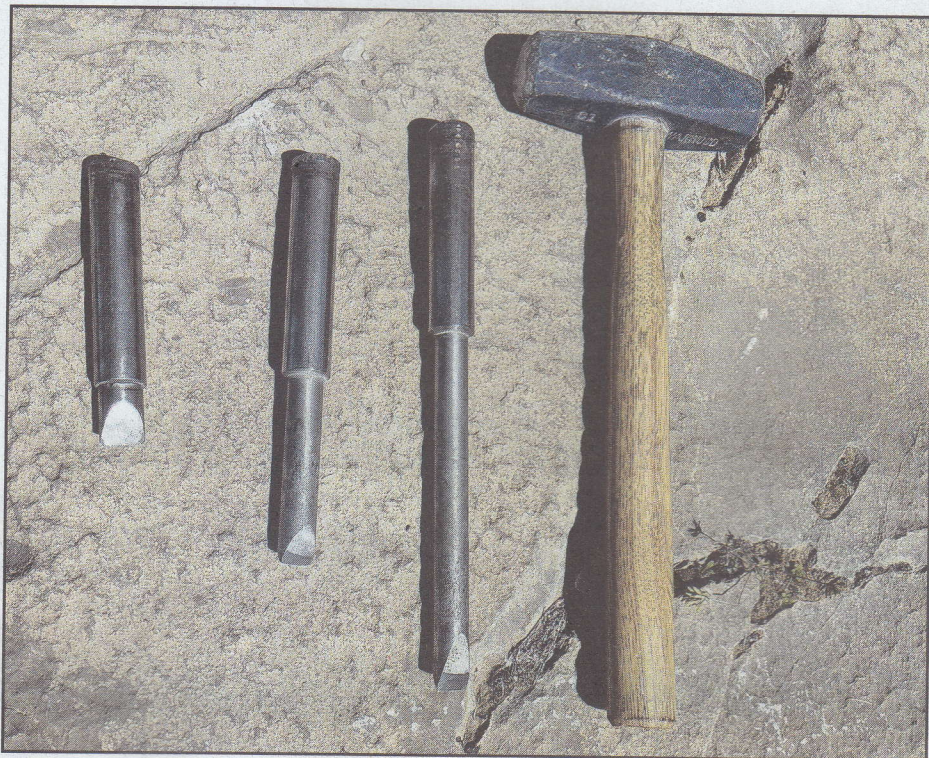
Close-up of the tools required for hand-drilling holes the way the old miners used to do it. The bit is rotated after each blow by the hammer.
