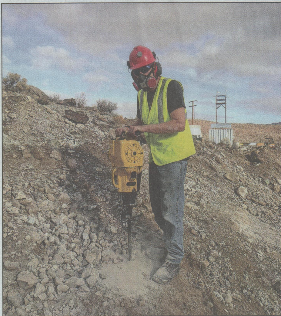
This motorized jackhammer drill is very handy for small mining operations, but the holes must be at least close to vertical because it's just too heavy to hold in a horizontal position and it cannot be used underground because of the exhaust fumes.
