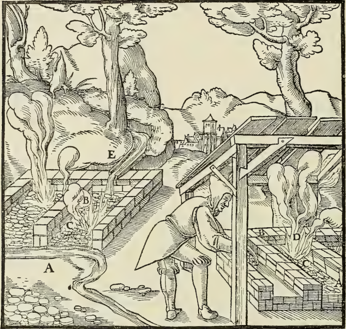
A—AREA. B—WOOD. C—ORE. D—CONE-SHAPED PILES. E—CANAL.
