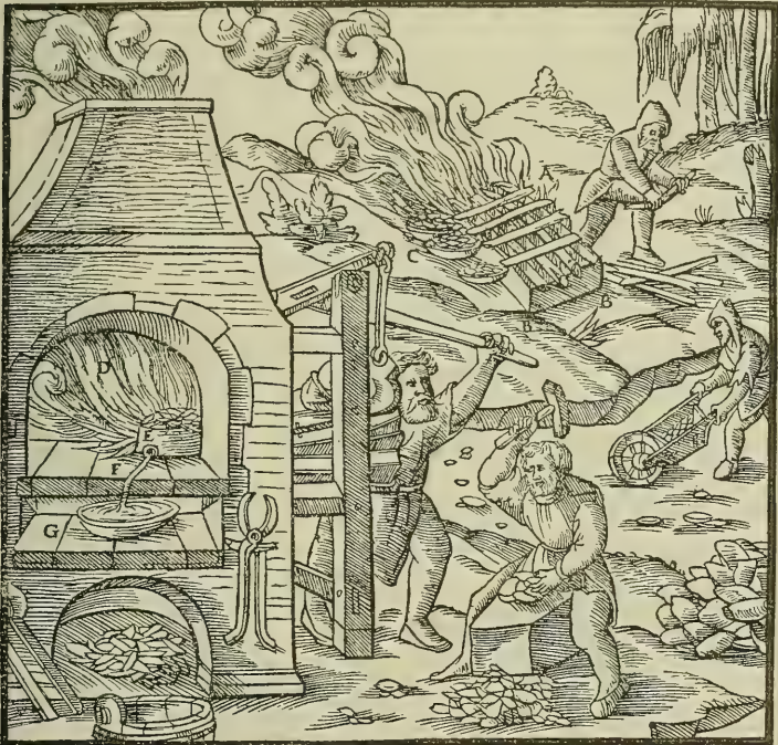
A—WOOD. B—BRICKS. C—PANS. D—FURNACE. E—CRUCIBLE. F—PIPE. G—DIPPING-POT.
