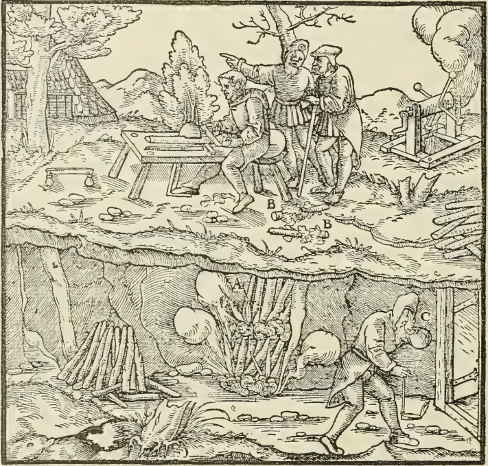
A—KINDLED LOGS. B—STICKS SHAVED DOWN FAN-SHAPED. C—TUNNEL.
