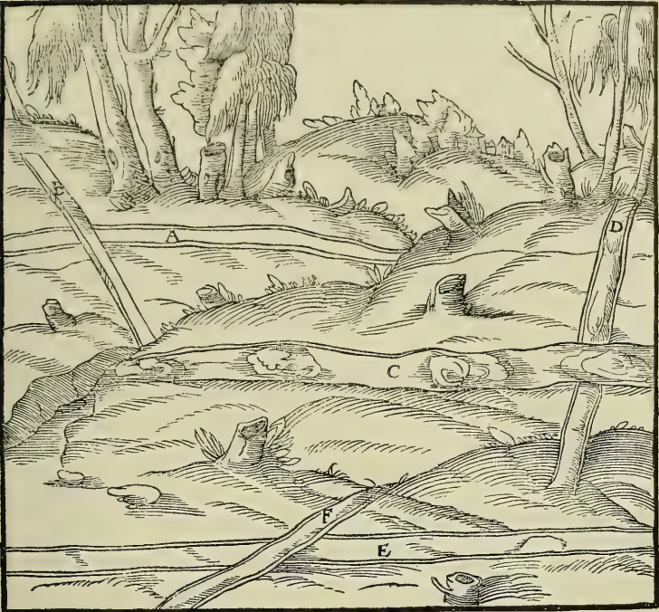
A—SOLID VEIN. B—SOLID STRINGER. C—CAVERNOUS VEIN. D—CAVERNOUS STRINGER. E—BARREN VEIN. F—BARREN STRINGER.
