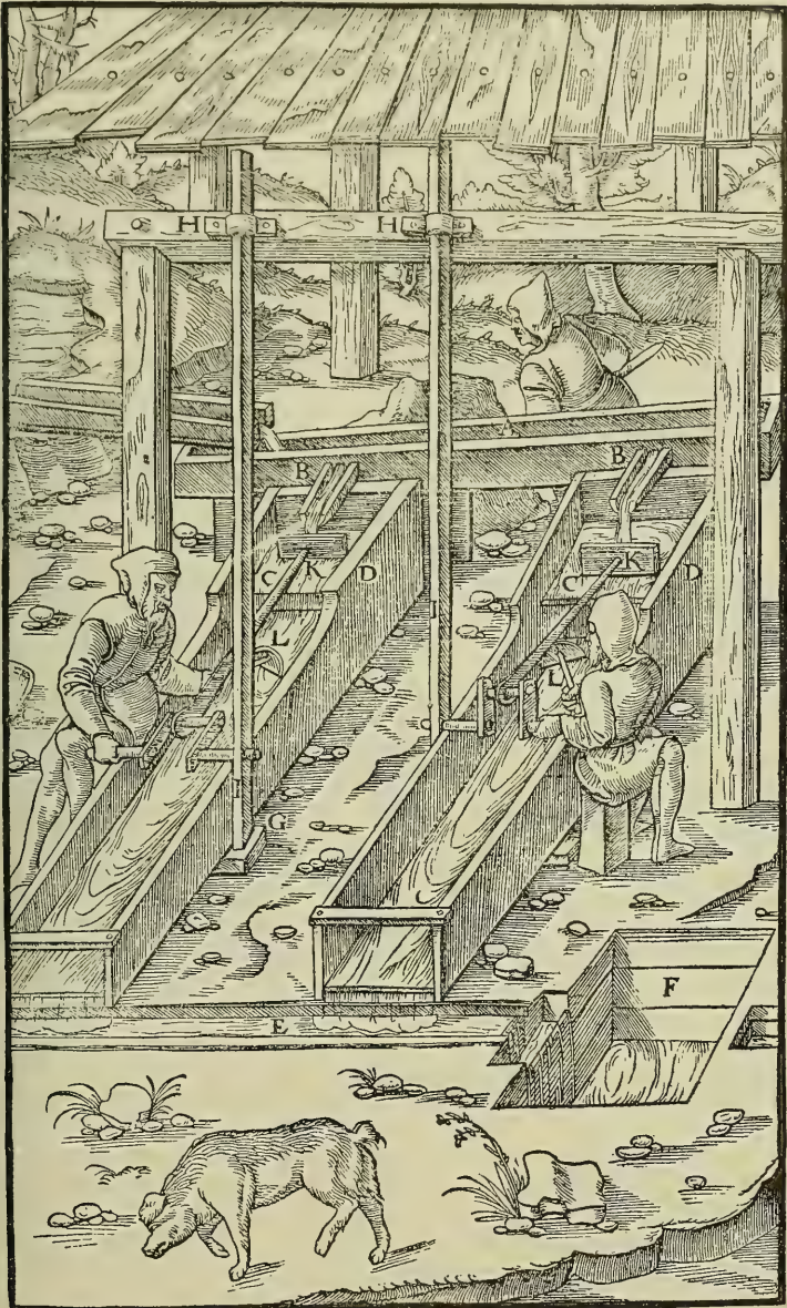
A—UPPER CROSS LAUNDRER. B—SMALL LAUNDERS. C—HEADS OF STRAKES. D—STRAKES. E—LOWER TRANSVERSE LAUNDRER. F—SETTLING PIT. G—SOCKET IN THE SILL. H—HALVED IRON RINGS FIXED TO BEAM. I—POLE. K—ITS LITTLE SCRUBBER. L—SECOND SMALL SCRUBBER.
