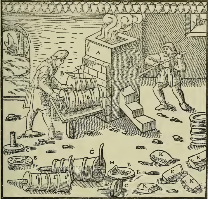
A—FURNACE. B—BELLOWS. C—IRON DISC. D—NOZZLE. E—WOODEN DISC. F—BLOW-HOLE. G—HANDLE. H—HAFT. I—HOOPS. K—MASSES OF TIN.
