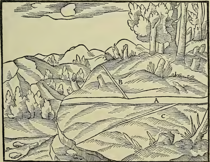
A—VEIN. B— Fibra incubens FROM THE SURFACE OF THE HANGINGWALL. C—SAME FROM THE FOOTWALL.
