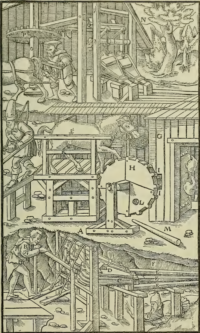
A—Machine first described. B—This workman, treading with his feet, is compressing the bellows. C—Bellows without nozzles. D—Hole by which heavy vapours or blasts are blown out. E—Conduits. F—Tunnel. G—Second machine described. H—Wooden wheel. I—Its steps. K—Bars. L—Hole in same wheel. M—Pole. N—Third machine described. O—Upright axle. P—Its toothed drum. Q—Horizontal axle. R—Its drum which is made of rundles.
