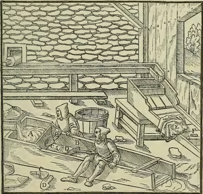
A—HEAD B—STRAKE. C—TROWEL. D—SCRUBBER. E—CANVAS. F—ROD BY WHICH THE CANVAS IS MADE SMOOTH.
