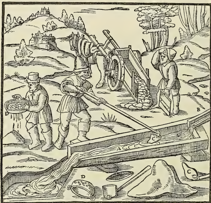
A—TROUGH. B—LAUNDER. C—HOE. D—SIEVE.
