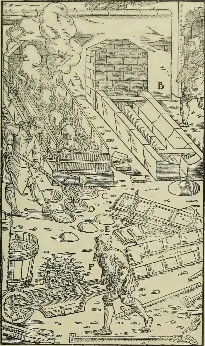
A — FURNACE IN WHICH THE OPERATION OF LIQUATION IS BEING PERFORMED. B — FURNACE IN WHICH IT IS NOT BEING PERFORMED. C — RECEIVING-PIT. D — MOULDS. E — CAKES. F — LIQUATION THORNS.
