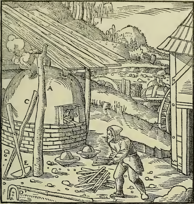
A—FURNACE. B—ITS MOUTH. C—POKER. D—RAKE WITH TWO TEETH. E—HOE.
