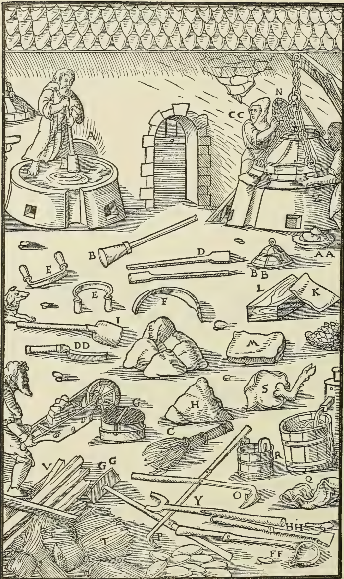
A—AN ARTIFICER TAMPING THE CRUCIBLE WITH A RAMMER. B—LARGE RAMMER. C—BROOM. D—TWO SMALLER RAMMERS. E—CURVED IRON PLATES. F—PART OF A WOODEN STRIP. G—SIEVE. H—ASHES. I—IRON SHOVEL. K—IRON PLATE. L—BLOCK OF WOOD. M—ROCK. N—BASKET MADE OF WOVEN TWIGS. O—HOOKED BAR. P—SECOND HOOKED BAR. Q—OLD LINEN RAG. R—BUCKET. S—DOESKIN. T—BUNDLES OF STRAW. V—WOOD. X—CAKES OF LEAD ALLOY. Y—FORK. Z—ANOTHER WORKMAN COVERS THE OUTSIDE OF THE FURNACE WITH LUTE WHERE THE DOME FITS ON IT. AA—BASKET FULL OF ASHES. BB—LID OF THE DOME. CC—THE ASSISTANT STANDING ON THE STEPS POURS CHARCOAL INTO THE CRUCIBLE THROUGH THE HOLE AT THE TOP OF THE DOME. DD—IRON IMPLEMENT WITH WHICH THE LUTE IS BEATEN. EE—LUTE. FF—LADLE WITH WHICH THE WORKMAN OR MASTER TAKES A SAMPLE. GG—RABBLE WITH WHICH THE SCUM OF IMPURE LEAD IS DRAWN OFF. HH—IRON WEDGE WITH WHICH THE SILVER MASS IS RAISED.
