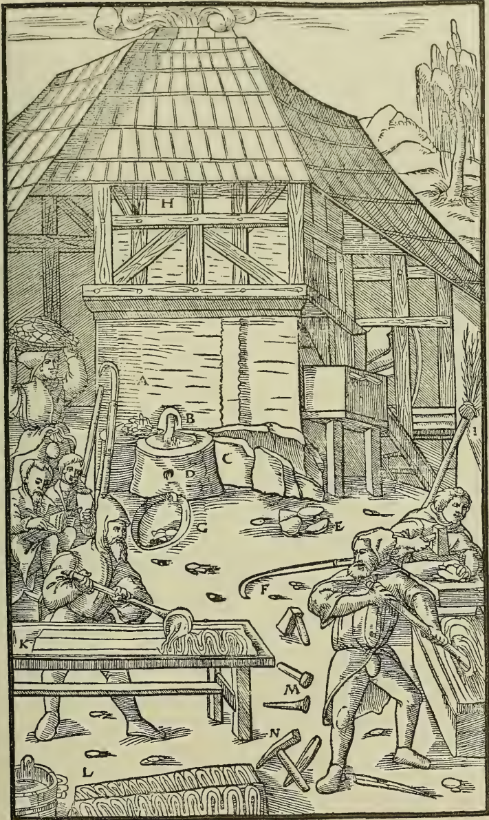
A—FURNACE. B—ITS TAP-HOLE. C—FOREHEARTH. D—ITS TAP-HOLE. E—SLAGS. F—SCRAPER. G—DIPPING-POT. H—WALLS OF THE CHIMNEY. I—BROOM. K—COPPER PLATE. L—LATTICEWORK BARS. M—IRON SEAL OR DIE. N—HAMMER.
