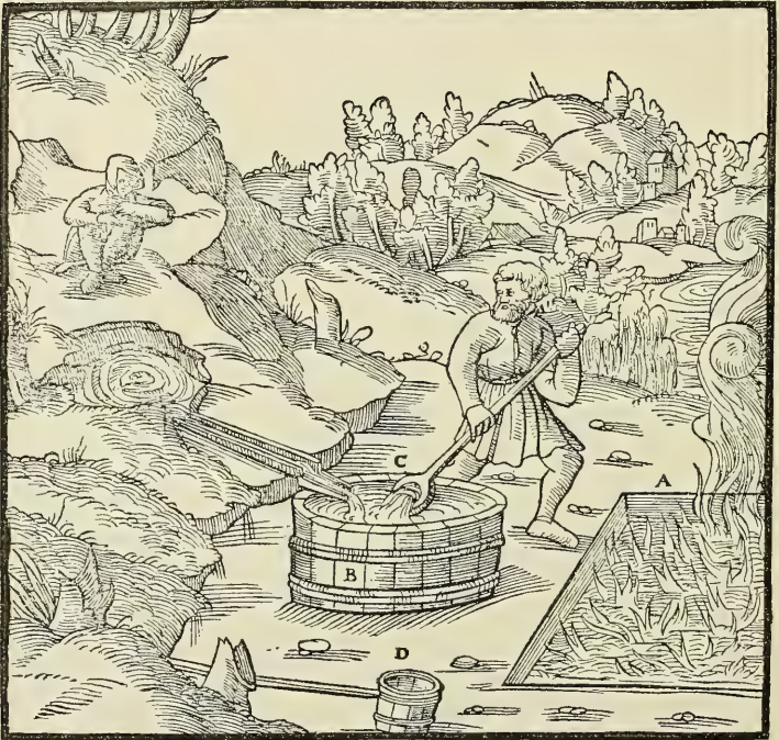
A—TRENCH. B—VAT INTO WHICH THE SALT WATER FLOWS. C—LADLE. D—SMALL BUCKET WITH POLE FASTENED INTO IT.
