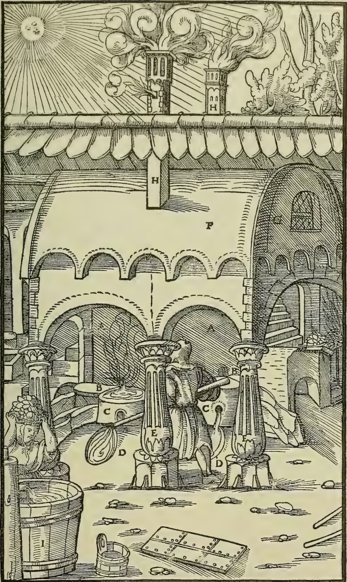
A—FURNACES. B—FOREHEARTH. C—THEIR TAP-HOLES. D—DIPPING-POTS. E—PILLARS. F—DUST-CHAMBER. G—WINDOW. H—CHIMNEYS. I—TUB IN WHICH THE COALS ARE WASHED.
