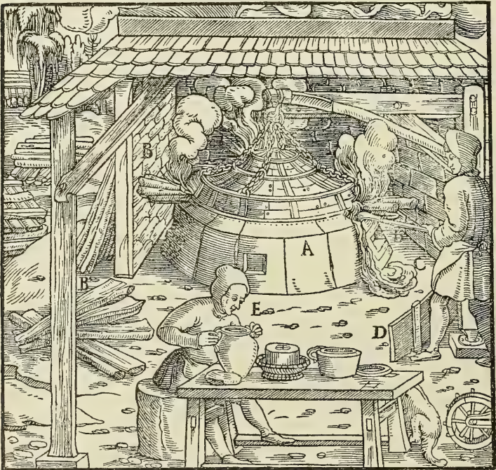
A—FURNACE. B—STICKS OF WOOD. C—LITHARGE. D—PLATE. E—THE FOREMAN WHEN HUNGRY EATS BUTTER, THAT THE POISON WHICH THE CRUCIBLE EXHALES MAY NOT HARM HIM, FOR THIS IS A SPECIAL REMEDY AGAINST THAT POISON.
