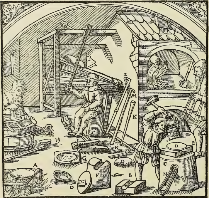
A—GRATE. B—BRASS BLOCK. C—BLOCK OF WOOD. D—CAKES OF SILVER. E—HAMMER. F—BLOCK OF WOOD CHANNELLED IN THE MIDDLE. G—BOWL FULL OF HOLES. H—BLOCK OF WOOD FASTENED TO AN IRON IMPLEMENT. I—FIR-WOOD. K—IRON BAR. L—IMPLEMENT WITH A HOLLOW END. THE IMPLEMENT WHICH HAS A CIRCULAR END IS SHOWN IN THE NEXT PICTURE. M—IMPLEMENT, THE EXTREMITY OF WHICH IS BENT UPWARDS. N—IMPLEMENT IN THE SHAPE OF TONGS.
