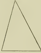
A TRIANGLE HAVING ALL ITS ANGLES ACUTE AND ITS THREE SIDES UNEQUAL.
