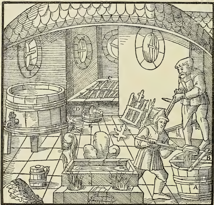
A—WOODEN TUB. B—CROSS-BARS. C—LATHS. D—SLOPING FLOOR OF THE CHAMBER. E—TUB PLACED UNDER IT.
